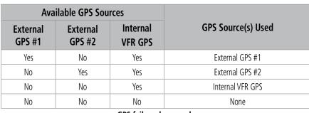
GPS failure downgrade
