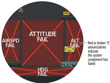
**Example of failure annunciations**
