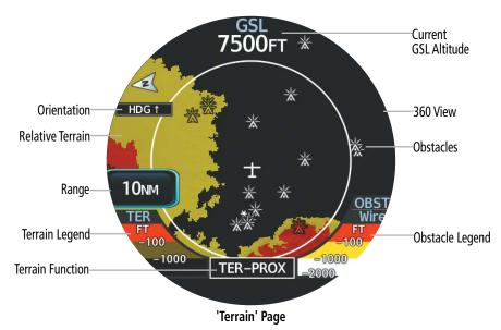
When Terrain-FLTA or TAWS-B data is available, potential impact areas will be indicated. If an obstacle and the projected flight path of the aircraft intersect, the display automatically adjusts the range setting to emphasize the display of the potential impact area.
