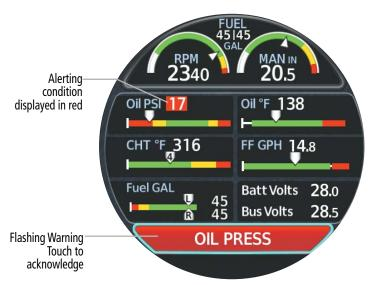
Flashing Oil Pressure Warning Annunciation
