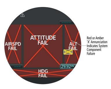
**Example of Failure Annunciations**
