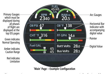
Gauges appearing as arc gauges on one page may appear as a vertical or horizontal bar on another. Exceptions include the Tachometer (RPM) and Manifold Pressure (MAN) Gauges which are always displayed as arc gauges. Other indications may display pointers, digital values, curves, or behavior bands.
